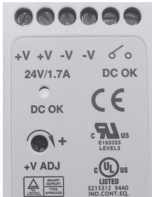
Figure 2: "DC OK" LED of DC Single Output Industrial DIN-rail Power Supply units.
